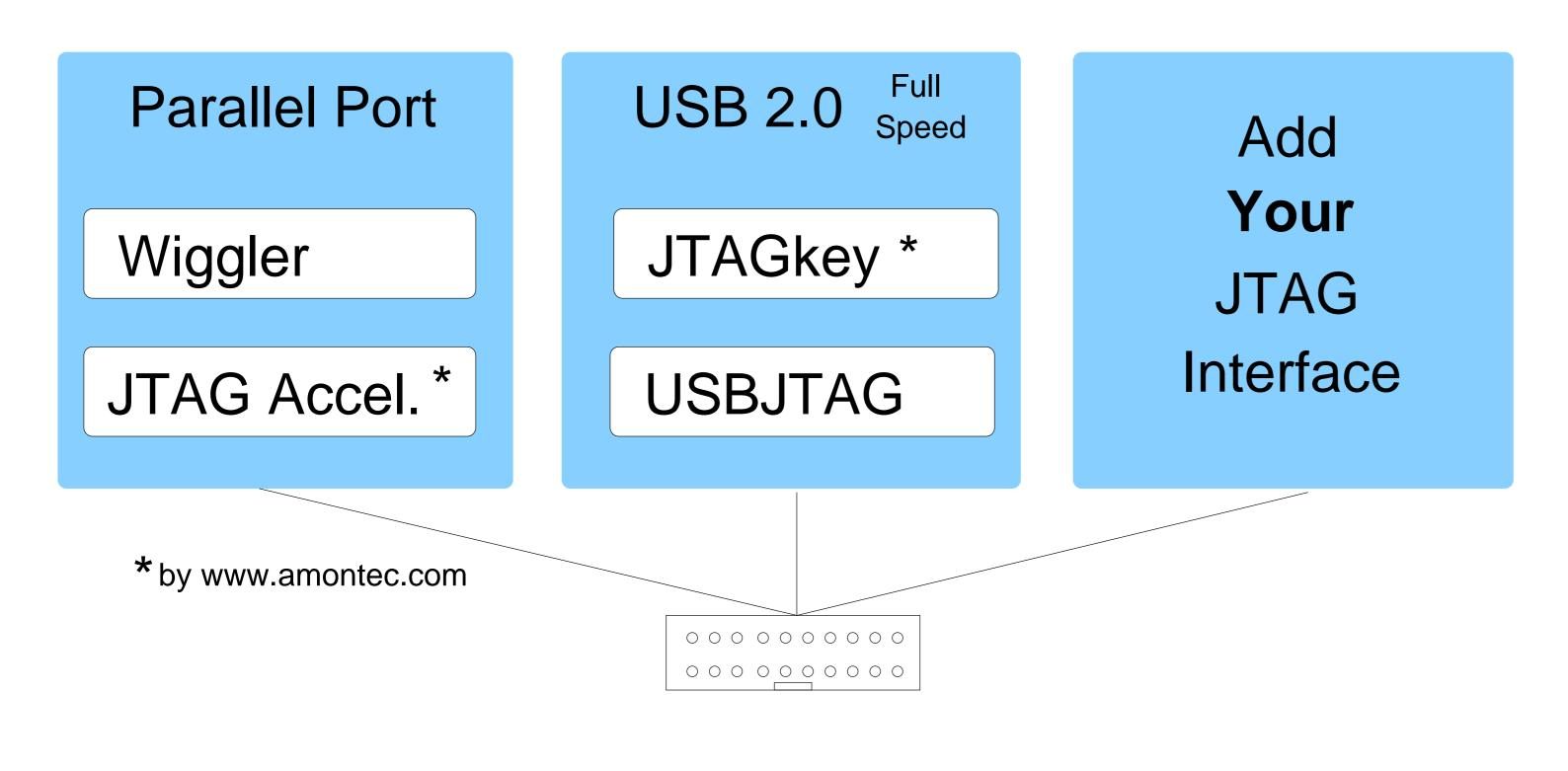
The interfaces in the **USB** group are all based on the **FT2232C** by FTDIChip [7]. You can easily add future interfaces, implemented e.g. by  $\mu$ **Cs with USB** full-speed interface (e.g. Atmel AT91SAM7S64), **USB 2.0 high-speed** interface (e.g. Cypress FX2), **TCP/IP** enabled devices, **FP-GAs** and so on.
